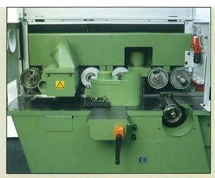
Both the near side and top head chipbreaker are of the Wadkin radial type ensuring maximum safety even with large variations in timber sizes. The radial chipbreaker allows the ultimate in control of thin or narrow sections and eliminates unevenness on the ends of the timber.
